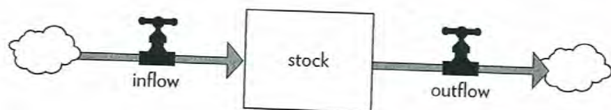
Figure 1. How to read stock-and-flow diagrams. In this book, stocks are shown as boxes, and flows as arrow-headed “pipes” leading into or out of the stocks. The small T on each flow signifies a “faucet;” it can be turned higher or lower, on or off. The “clouds” stand for wherever the flows come from and go to—the sources and sinks that are being ignored for the purposes of the present discussion.
